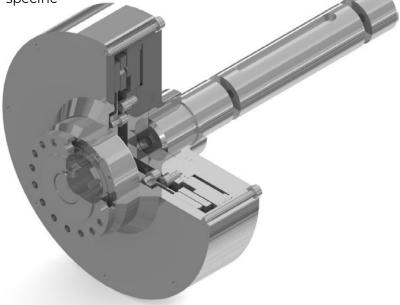
When compressed air is applied to the piston, the piston moves the pressure plate against the rotor and in this manner transfers the torque. When the compressed air is relieved, a spring pulls the piston with the pressure plate back to the starting position. The driven auxiliary unit is no longer in motion.
